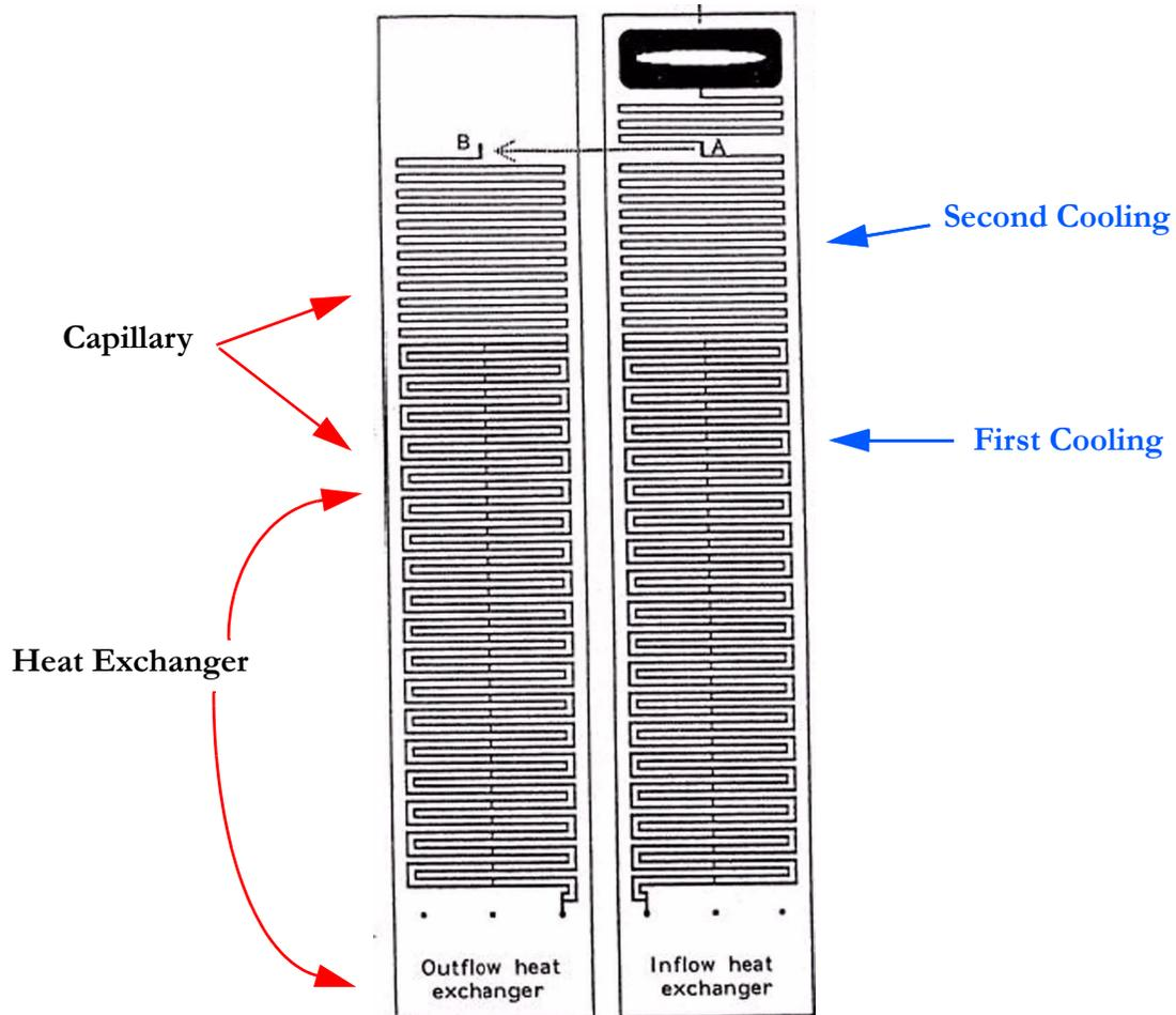
**FIGURE 2. The heat exchangers found in a Joule Thomson refrigerator.**
