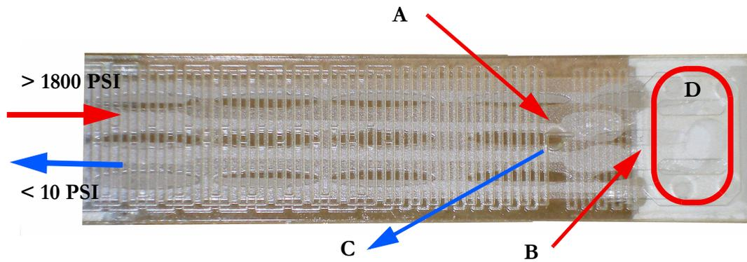
**FIGURE 3.** The channels in the Joule Thomson refrigerator channel the high pressure gas. For further information on the fabrication of these refrigerators, please refer to W.A. Little, Review of Scientific Instruments 55, 661 (1984).
